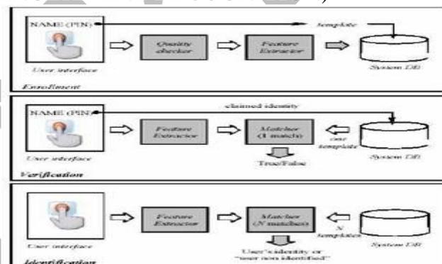
This is the block diagram of the enrollment, verification and identification systems are depicted. 4 modules are used in this biometric system.
